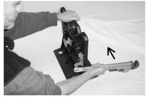
**D.** Hold the wrench in a horizontal position with <u>jaws</u> facing <u>up</u> and coming from behind the Rack-A-Tier. See diagram.
