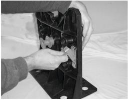
**B.** Insert the HOOKER body into the Rack-A-Tier handle and reinstall the slide The tool rest just pushes into the centre hole of the Rack-A-Tier. It can be stored in any of the five holes. See diagram.
