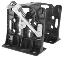
**G.** To engage the pipe, rotate the wrench up, place the pipe in the "V notch" and drop the wrench onto the pipe. With the jaws correctly adjusted to the work, gravity will lock the wrench in place. See diagram.
