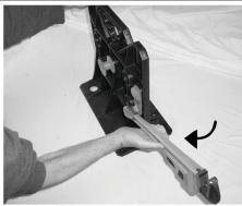
**E**• Slip the key hole on the wrench handle over the hook and manoeuvre the wrench around until it is at the front of the Rack-A-Tier. See diagram.
