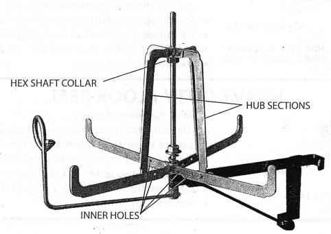
RELOCATE HUB SECTIONS TO THE INNER HOLES.
