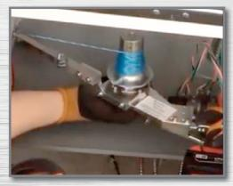
Tight quarter pulling in ceiling-mounted junction boxes inside joists are made easy with the CP1000. Let the puller do the work!
