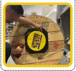
Flip the reel over so that it's now resting on the Tug Wise. The Tug Wise Standard has 1000 lb. carrying load for wood and plastic reels.
