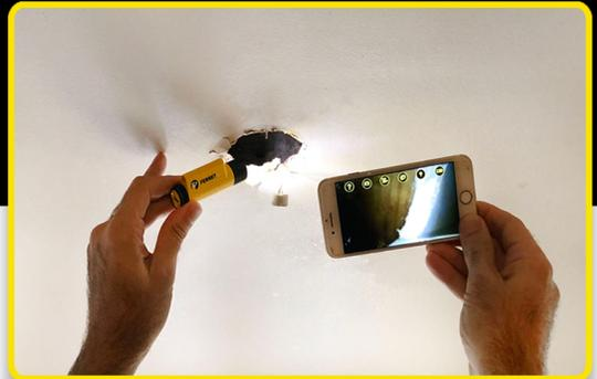
**Wire Fishing:** If your job requires you to fish wire, this is the best tool investment you will ever make. The included hook and magnet attachments are perfect for wire fishing. With the included hook you can navigate right to the wire you want and pull it out. Being able to get eyes inside the wall while you are fishing is a game changer.
